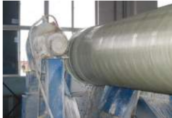
Trimming and de-molding
