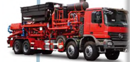
Fracturing Pumping Equipment 1#
