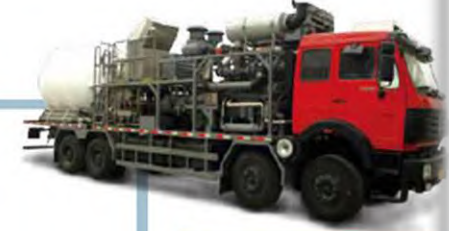
Nitrogen Pumping Equipment
